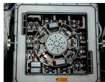
The T-Cell Activation in Aging investigation will use the Kubik incubator aboard the International Space Station. This image shows similar sample units from a previous study
